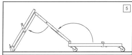
Subsequently, the load arm and the stand are connected with the locating pin.
