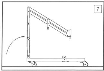
For reinforcement two props are put over the fork-bolt of the underframe and the stand.
