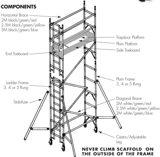
MAX SAFE WORKING LOAD FOR STRUCTURE 750KG MAX SAFE WORKING LOAD FOR PLATFORM 250KG
