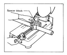
If you use a spacer block which is slightly narrower than the workpiece as shown in the figure, you can also utilize the wheel economically.
