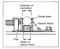
Long workpieces must be supported by blocks of non-flammable material on either side so that it will be level with the base top.
